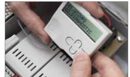
DYL handheld programmer with display for easy programming
